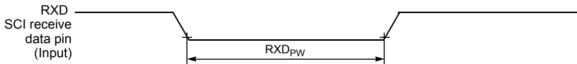
Figure 10-16 RXD Pulse Width
