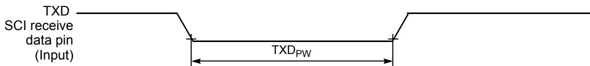
Figure 10-17 TXD Pulse Width
